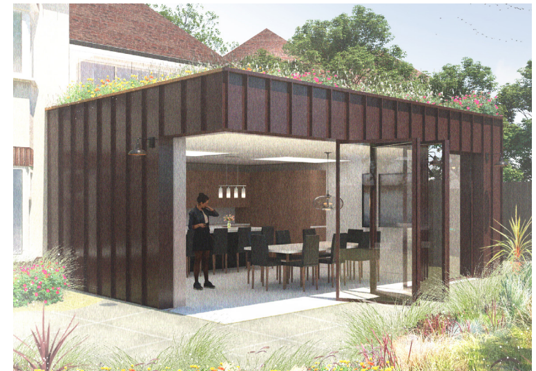
55 WA benefits from ASHP, new insulation, and a biodiverse roof.
